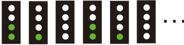
Discharging indication if SOC=50%
