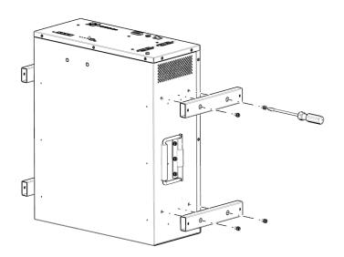
4. Screw the 4 connectors to the holders with TM4\*8 screws.
