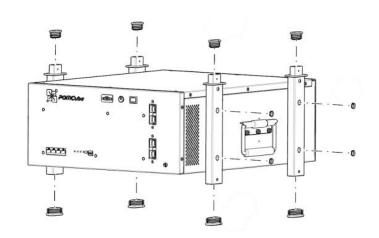
6. If you need to stack-up batteries, no square inner plugs are needed for the upper battery. Screw the holders into connectors.
