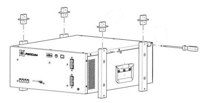
Install the square inner plugs and screw hole plugs accordingly.
